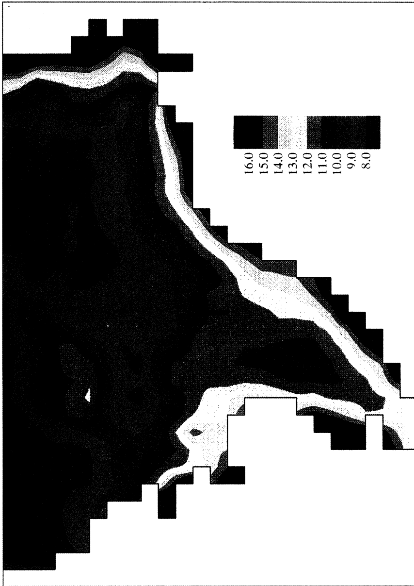
Figure 2. Sea-bed temperature, 2 June 1989, after two months integration of three-dimensional prognostic model from well-mixed conditions. The developed front can be seen extending from northeast England to the north Dutch and German coasts.
